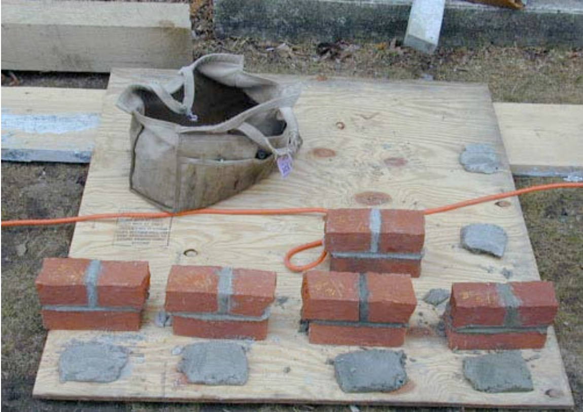
Figure 33 and 34: Mortar samples were made up by the mason for LPC approval based on the mortar analysis report provided by Jablonski-Berkowitz Conservation in New York. While the color and texture were matched, the hardness was made to be compatible with the new brick selected to face the pedestals.
